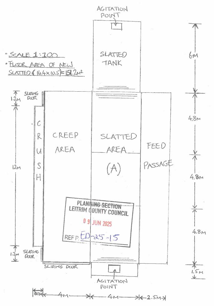
FLOOR PLAN OF PROPOSED SLATTED SHED(A)
