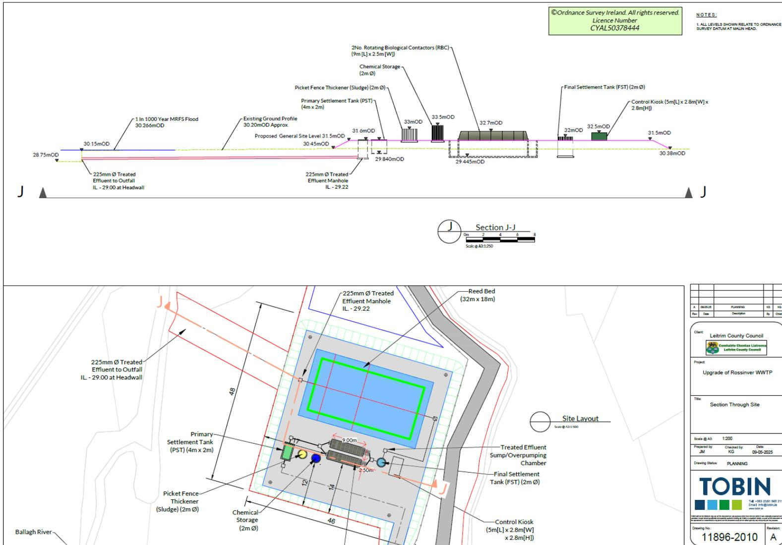
Figure 1. Drawing 11896-2010 location of sump / overpumping chamber which will take over in the event of an extreme flood event, as supplied by TOBIN Ltd. (not to scale).
