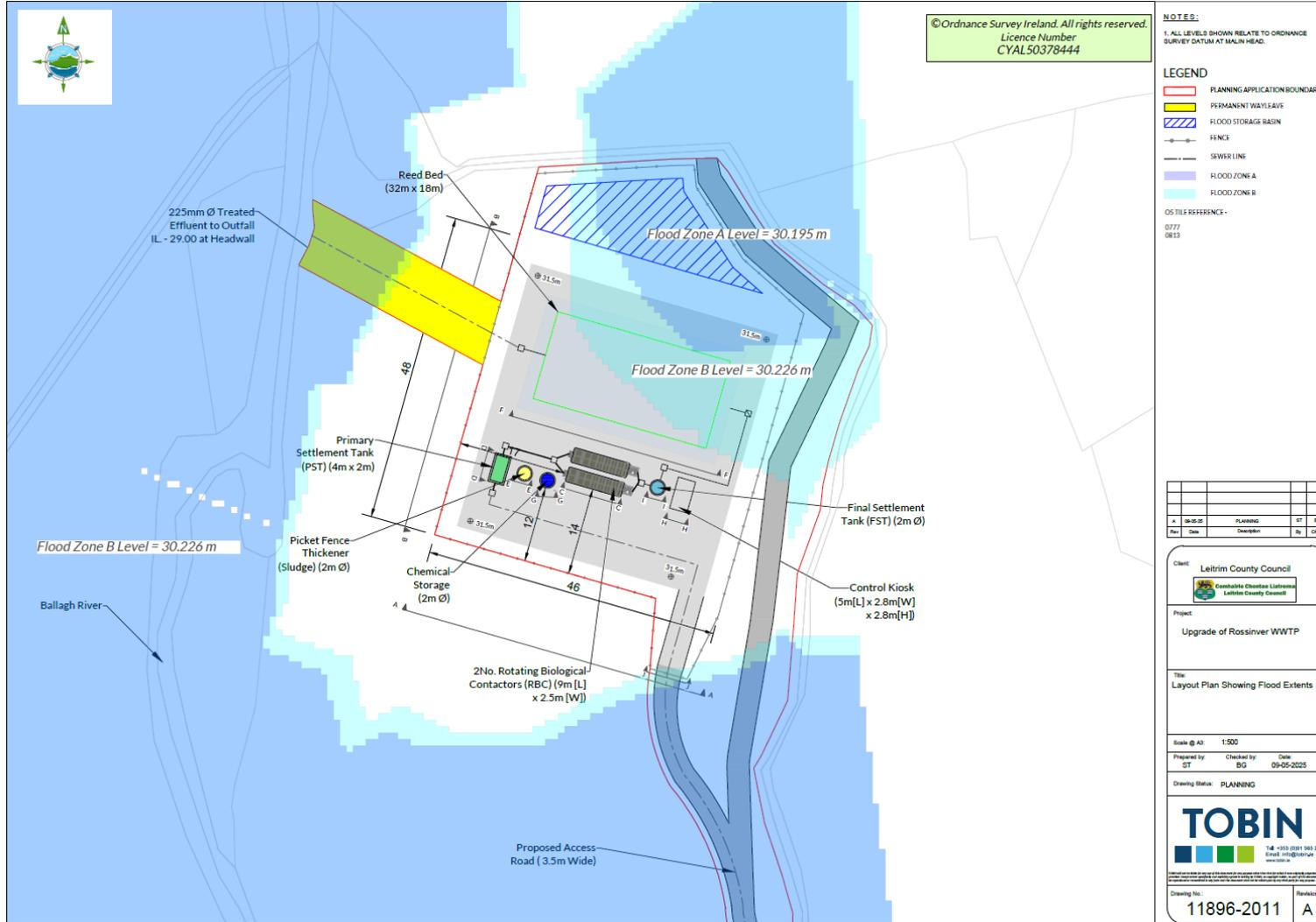
Figure 2. Drawing 11896-2011 Flood extents at the project location as supplied by TOBIN Ltd. (not to scale).
